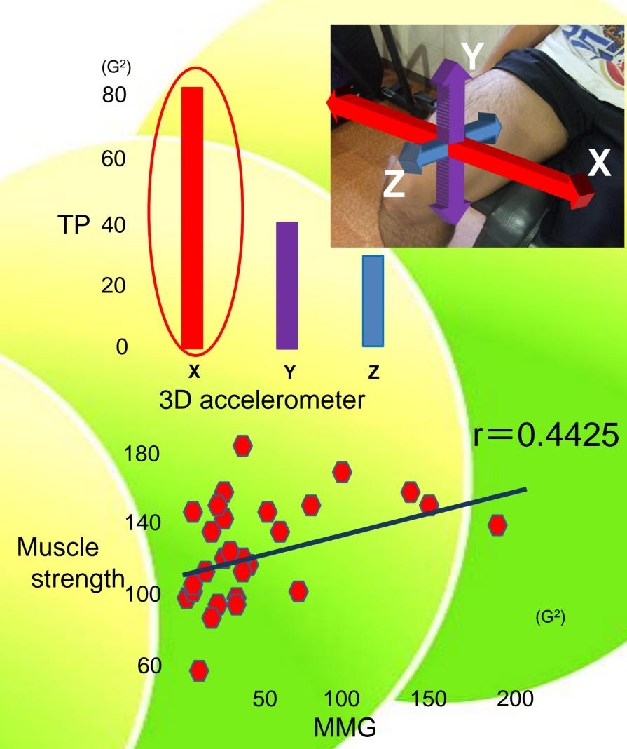
The maximum mechanical vibrations were obtained in the horizontal direction.
